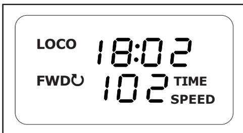
Only the Master Cab (Cab #1) can program the time, time ratio, and AM/PM or military (24 hr) time. The time settings entered by the Master Cab are stored in the Prodigy Wireless DCC system base unit memory. The settings will remain unchanged until you reprogram them. The time is sent to all Cabs operating on the layout so railroad schedules can be maintained.
