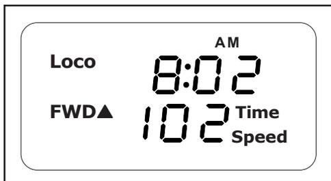
The left LCD display shows time of 8:02AM. The current loco is moving forward at a speed of 102.
