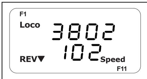
The left LCD display shows that the current loco is 3802 running in reverse at a speed of 102. Its accessory functions F1 and F11 are on.
