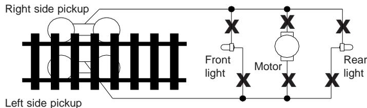
Figure 2 shows you how to wire the decoder. After disconnecting the motor terminals from pickups, connect the red wire to the right side pickup and the black wire to the left side pick up. Connect the orange wire to the motor terminal that originally connect to the right pickup. Connect the gray wire to the motor's other terminal. Connect the front light to the blue wire and the white wire. Connect the rear light to the blue wire and the yellow wire.
