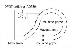
Before a loco crosses the first insulated gap you must make sure the polarity of reverse loop section and Main Track are matched at the first gap. If not flip the switch. Otherwise it will cause a short circuit. After the loco passes the first gap completely, you need to change the polarity of the reverse loop section by flipping the switch so that the polarity of the reverse loop section and Main Track are matched at the second gap.
