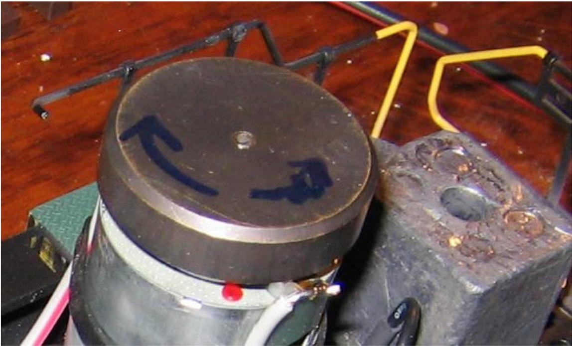
Using the bottom of a plastic craft paint container, I fashioned a thin baffle for the speaker. The speaker with baffle was then hot glued into the fuel tank casting. The speaker wires were also lengthened at this time to afford more flexibility in the final placement of the decoder. Before the fuel tank casting was attached to the chassis, I placed some foam rubber on top of the speaker to add a little bass to the sounds, and routed the speaker wire with plug up through the chassis.
