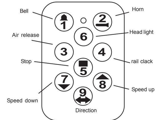
Note: The transmitter operates on a 12V (A123) battery, readily found in most stores that sell electronic equipment.
