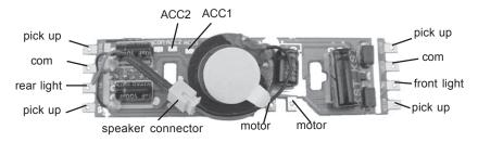
The motor terminals must be isolated from the wheel pickups. The four pickup wires go to pickup tabs. The motor wires go to motor tabs.
