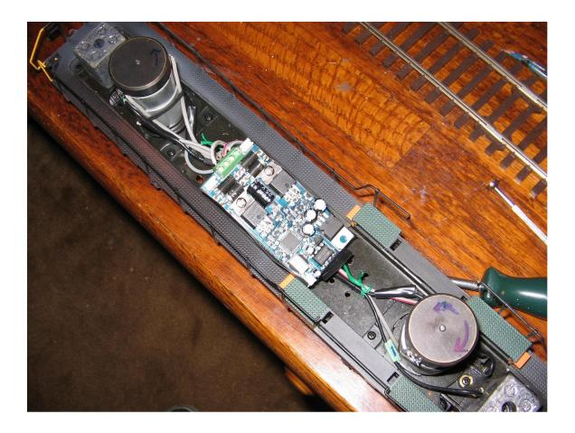
The wires were then neatly bundled with wire ties and the decoder installation was finished except for plugging in the headlights, and re-installing the body shell.
