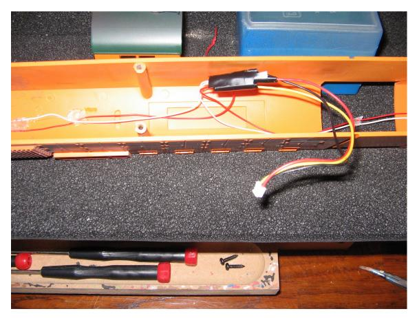
The cab was left off to check inside the shell that nothing was pinched or rubbing against the flywheels or the decoder.
