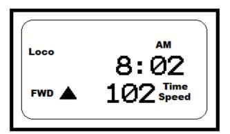
The above LCD display shows time of 8:02AM. The current loco is moving forward at a speed of 102. The back-lit display on the Prodigy Elite base unit will always show the present time on the fast clock.
