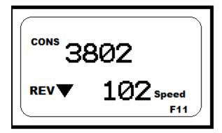
The above LCD display shows a Universal Consist group led by lead loco 3802 running in reverse at a speed of 102.
