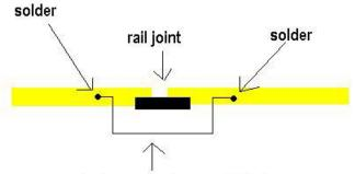
wire jumper between rail joints to compensate for loose or corroded rail joiners
