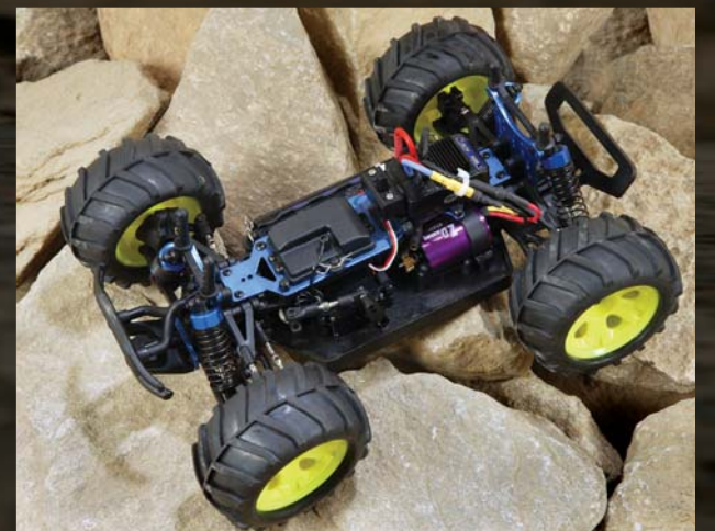
The chevron-tread tires are a dead giveaway that this is the monster-truck chassis. The trucks also have larger bumpers that offer more protection than the buggy bumpers do.
