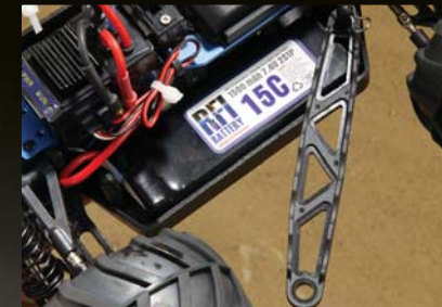
With a LiPo battery, you get solid performance from beginning to end. The included 1500mAh RFI battery is good for about 15 minutes of continuous running.
