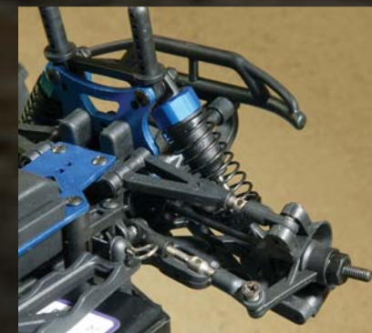
The suspension's thick turnbuckles allow easy adjustments and should withstand quite a bit of abuse.
