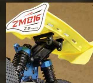
The wing is on an adjustable mount—just like the bigger cars.
